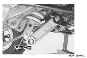
Install the cushion rod and cushion lever. Refer to "Cushion Rod / Cushion Lever Removal and Installation (Page 2C-7)".
