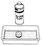
Apply the brake fluid to piston seal (4) and dust seal (5).
