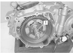
Install the generator rotor (2). Refer to "Generator Removal and Installation in Section 1J (Page 1J-5)".
