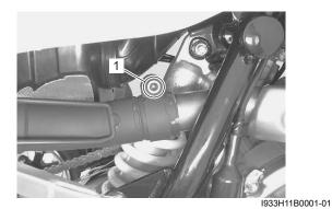
2) Remove the muffler (2) by removing the mounting bolts.
