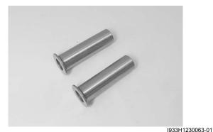
3) Install the spacers. Refer to "Swingarm Dust Seal / Bearing Removal and Installation (Page 2C-14)".
