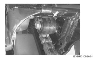
**Drive Chain Roller Removal and Installation**
